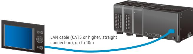
LAN cable (CAT5 or higher, straight connection), up to 10m
