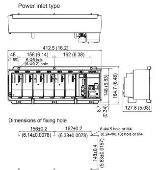
Unit: mm (approx. inch) Unless otherwise specified, tolerance is  $\pm 3\%$  (however, tolerance is  $\pm 0.3$  mm when below 10 mm).
