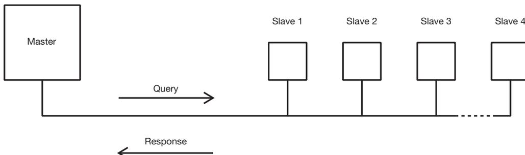
In the MODBUS Protocol the master can address individual slaves, or, using a special "Broadcast" address, can initiate a broadcast message to all slaves. The SKD-005-M Digital meter do not support the broadcast address.
