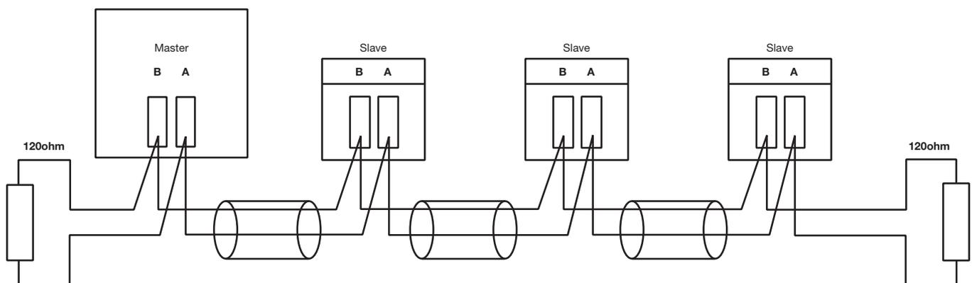
There must be no more than two wires connected to each terminal, this ensures that a "Daisy Chain or "straight line" configuration is used. A "Star" or a network with "Stubs (Tees)" is not recommended as reflections within the cable may result in data corruption.
